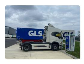
**Electric Truck in France:** since January 2024, an eTruck commutes daily between the two GLS hubs in Paris. To support this, GLS France has outfitted the Paris-Sud hub with a 360 kW charging station, ensuring efficient charging for the eTruck.
